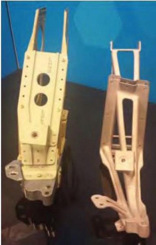
Conventionally machined bracket assembly (left) and redesigned 3D-printed bracket (right), courtesy of Airbus
