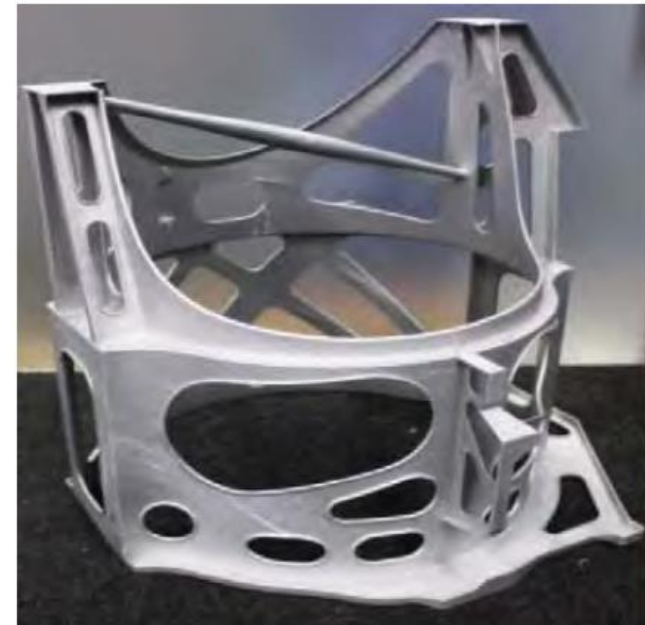
AM-produced hydraulic reservoir rack consolidates 126 parts into one, courtesy of Airbus
