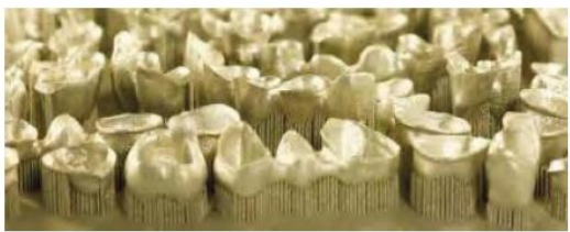
3D-printed dental copings, courtesy of Concept Laser
