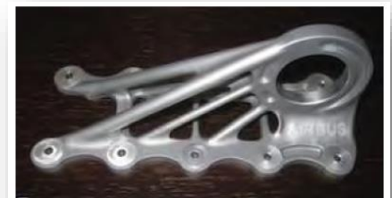
Cabin bracket for the A350 made with powder bed fusion, courtesy of Airbus
