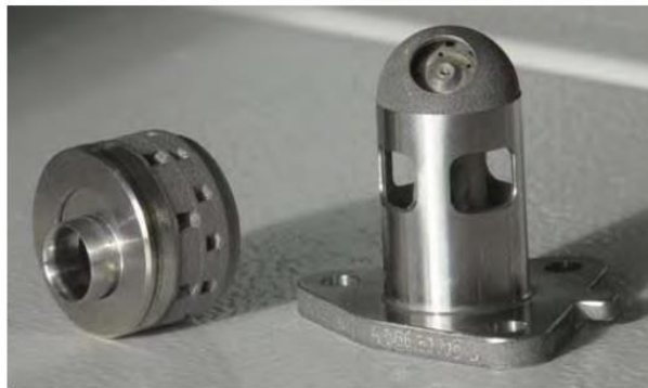
Combustor swirler and injector nozzle parts made by AM, courtesy of Turbomeca
